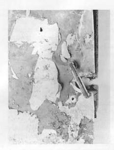
Part of the door leading from the passenger compartment into the main deck cargo compartment. The door was blistered, partly collapsed and splattered with an unidentified blue substance on the cargo compartment side. Crew would have entered the cargo compartment through this door to inspect the fire and attempt to bring it under control
