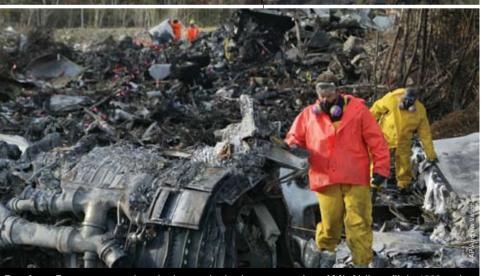
**Break up:** Emergency workers look over the broken up remains of Mk Airlines flight 1602 at the accident site near Halifax, Nova Scotia, Canada. Eye witnesses said that the takeoff seemed normal until the last minute when they saw the 747's tail hit the earthen mound supporting the ILS and the aircraft's tail break off.
