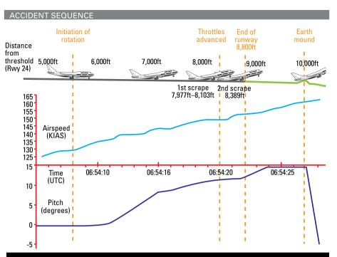
**Tail scrape:** The 747's tail scraped the runway twice before the aircraft hit an earth mound at the end of the runway after failing to achieve takeoff performance.
