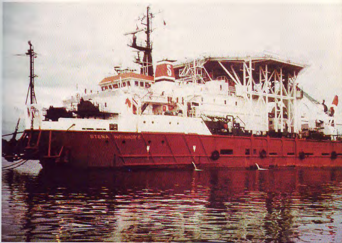
The Stena Workhorse, a large motor vessel designed to support offshore oilfield work, was the mothership which supported the ROV operation during the search and recovery phase. Its large open aft workdeck was ideal for the temporary stowage of debris brought to the deck by four cranes (DCA)
